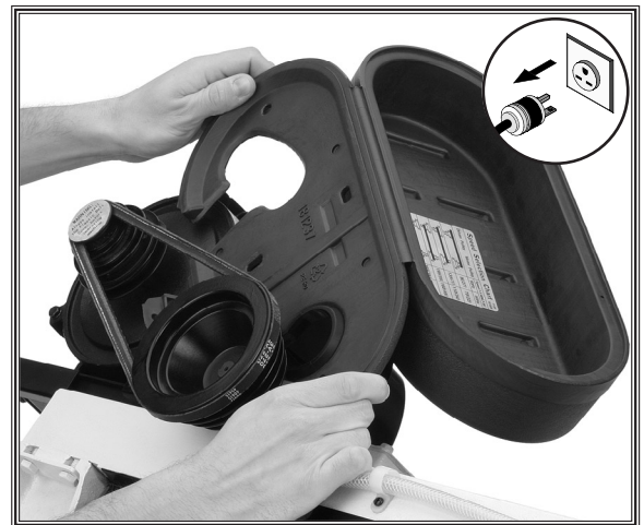
Figure 19. Positioning the pulley cover.
